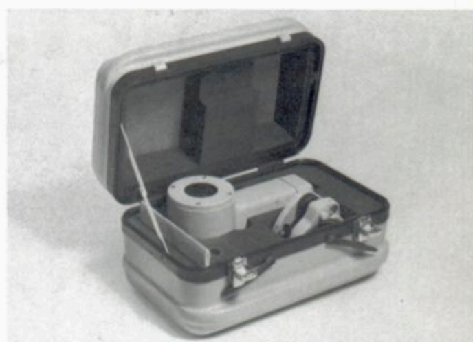
Optical plummet in the container
